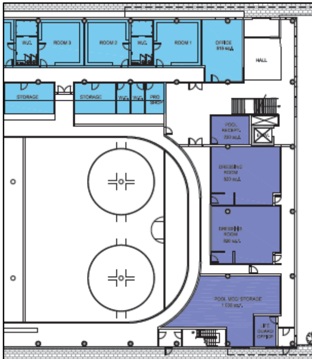
1 st floor: Space for pool offices and dressing rooms, hockey dressing rooms, elevator
